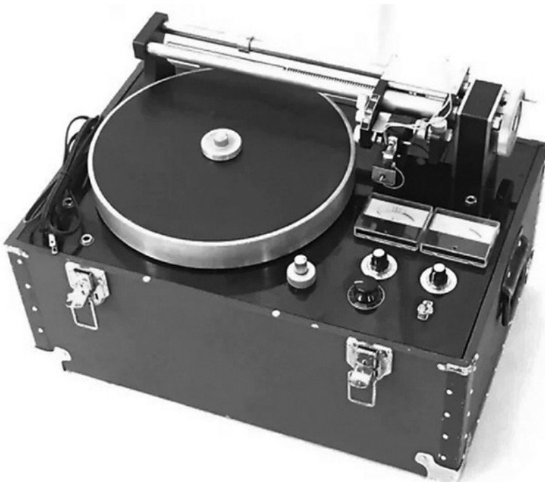
Figuur 1. Apparaat waarop de bone music platen werden gekopieerd (bron: atlasrecords.co.uk/blogs/all-about-vinyl/bone-music-or-music-on-ribs-how-to-share-music-in-a-totalitarian-state ).
